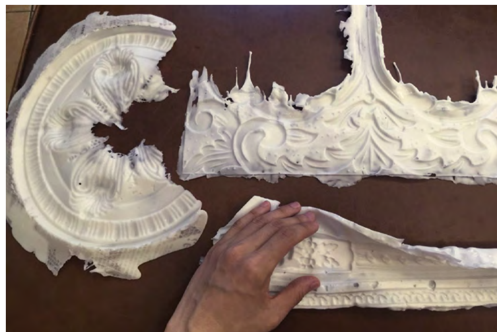
fig.38.1-3 Rongkai He put silicone on the surface of some furniture to copy the decoration.
