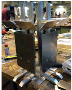
fig.43.2 The aluminium structure of the base.
