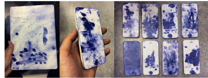
fig.41-42 Top: fingerprints left on the touch screen after using the devices for a few hours. Bottom: Later, baby powder was used to capture the fingerprints which were then scanned and adjusted into patterns.
